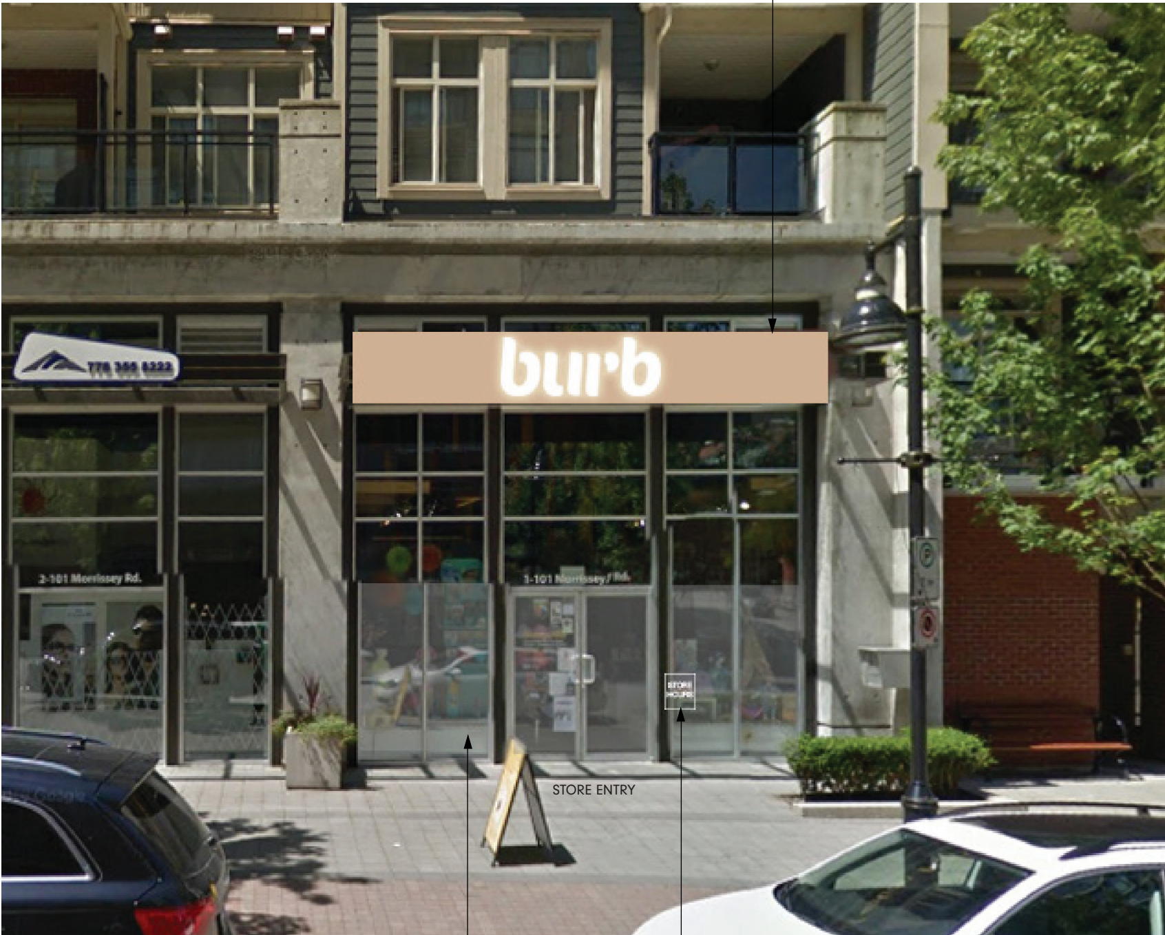
PIN-MOUNTED CHANNEL LETTER ILLUMINATED STOREFRONT SIGN, WHITE POWDER COATED METAL ON POWDER COATED METAL BACKING
