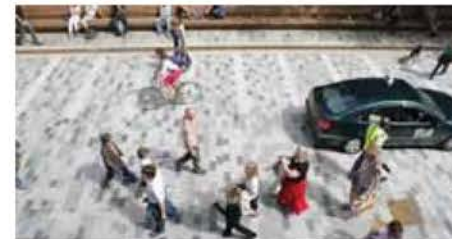
Paving bands to be oriented along the North-South axis, perpendicular to Spring Street paving pattern on private property to complement Spring Street patterns.
