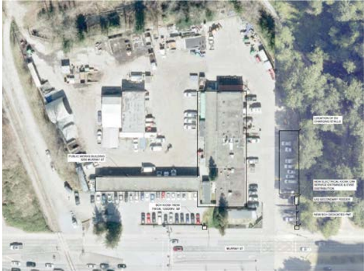
Figure 6: Public Works proposed electrical infrastructure site plan
