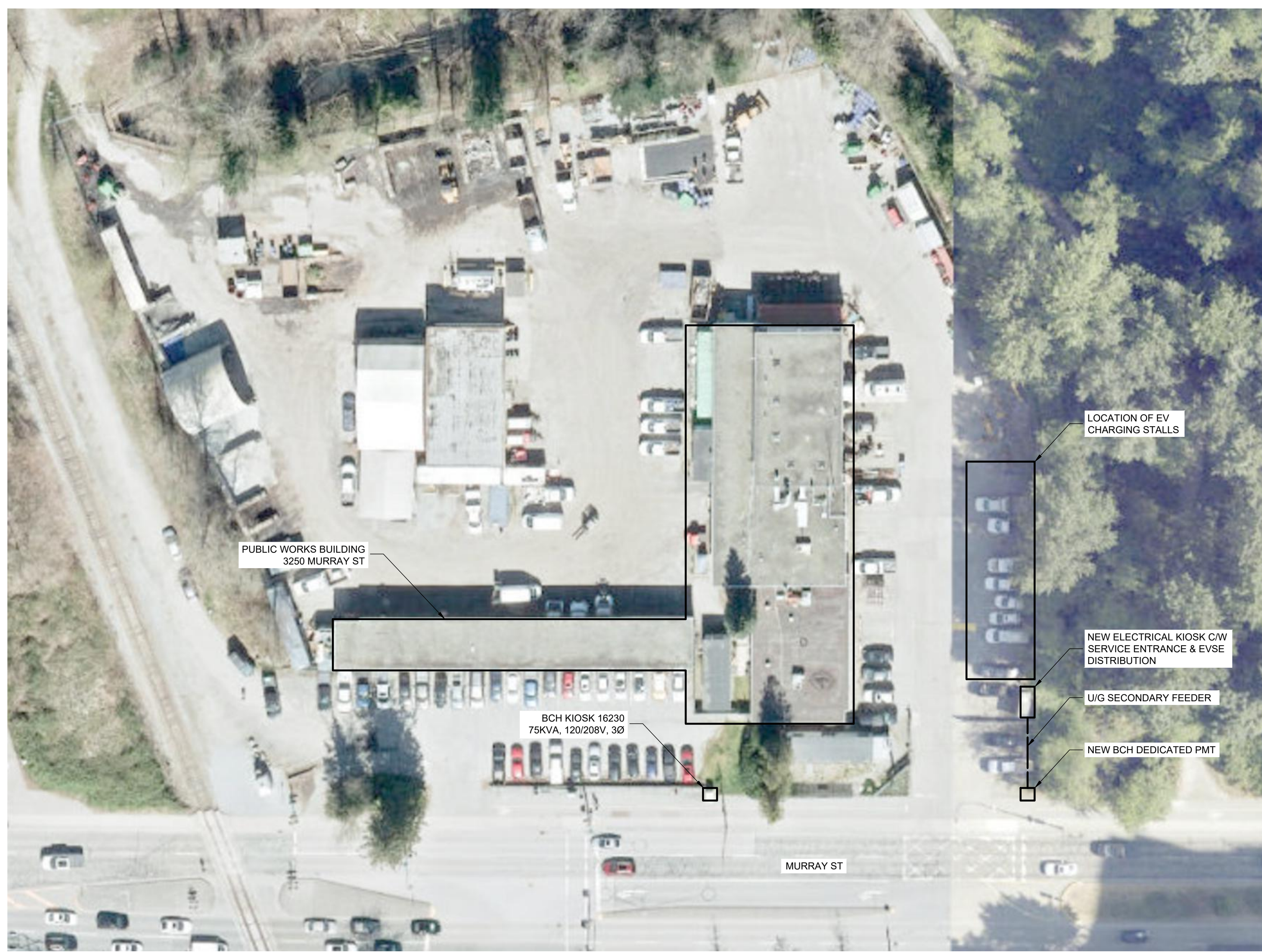
DETAIL 1 SITE PLAN 1:400 PUBLIC WORKS YARD
