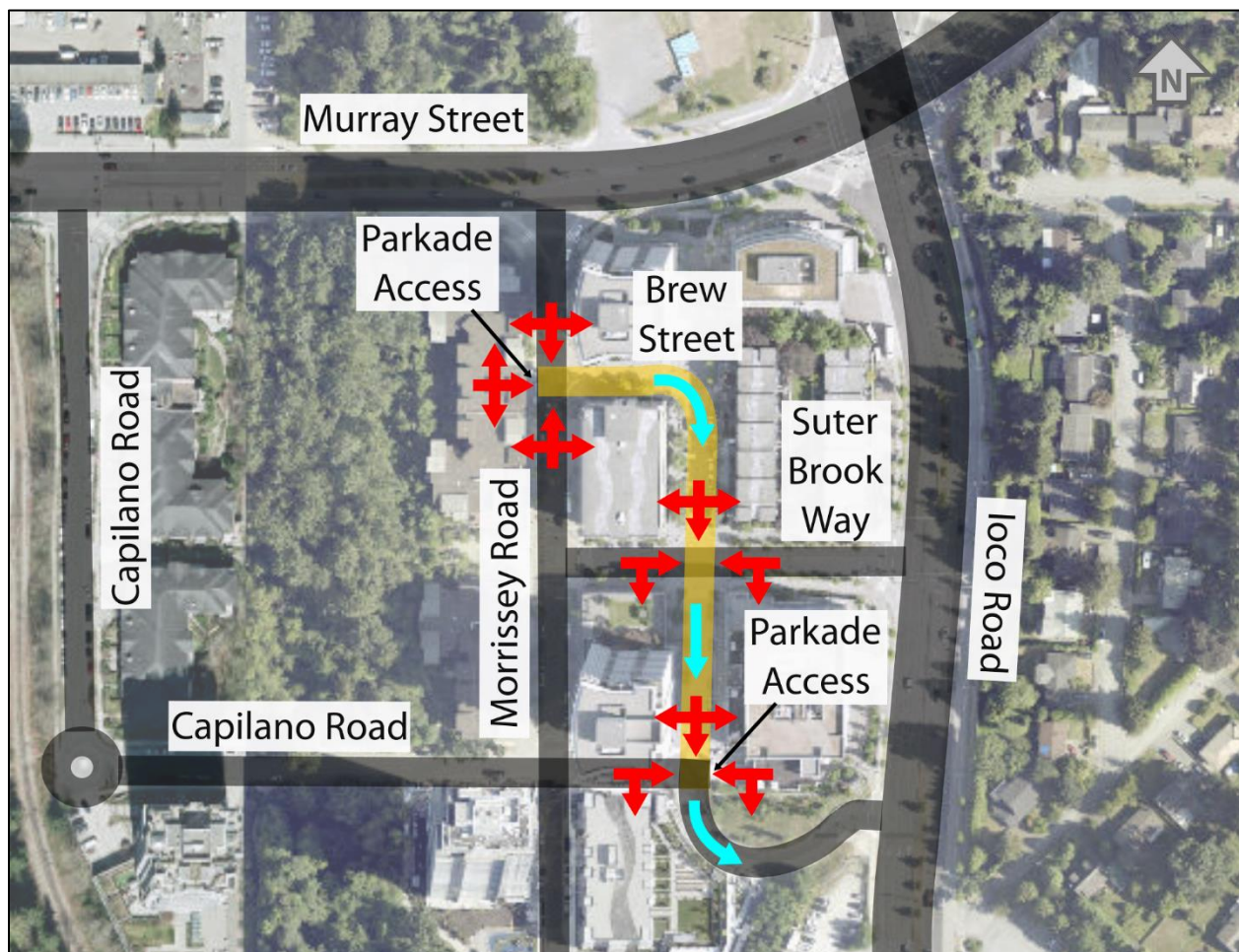
Figure 4-1: Brew Street One-way Traffic Conditions as Observed in March 2023
