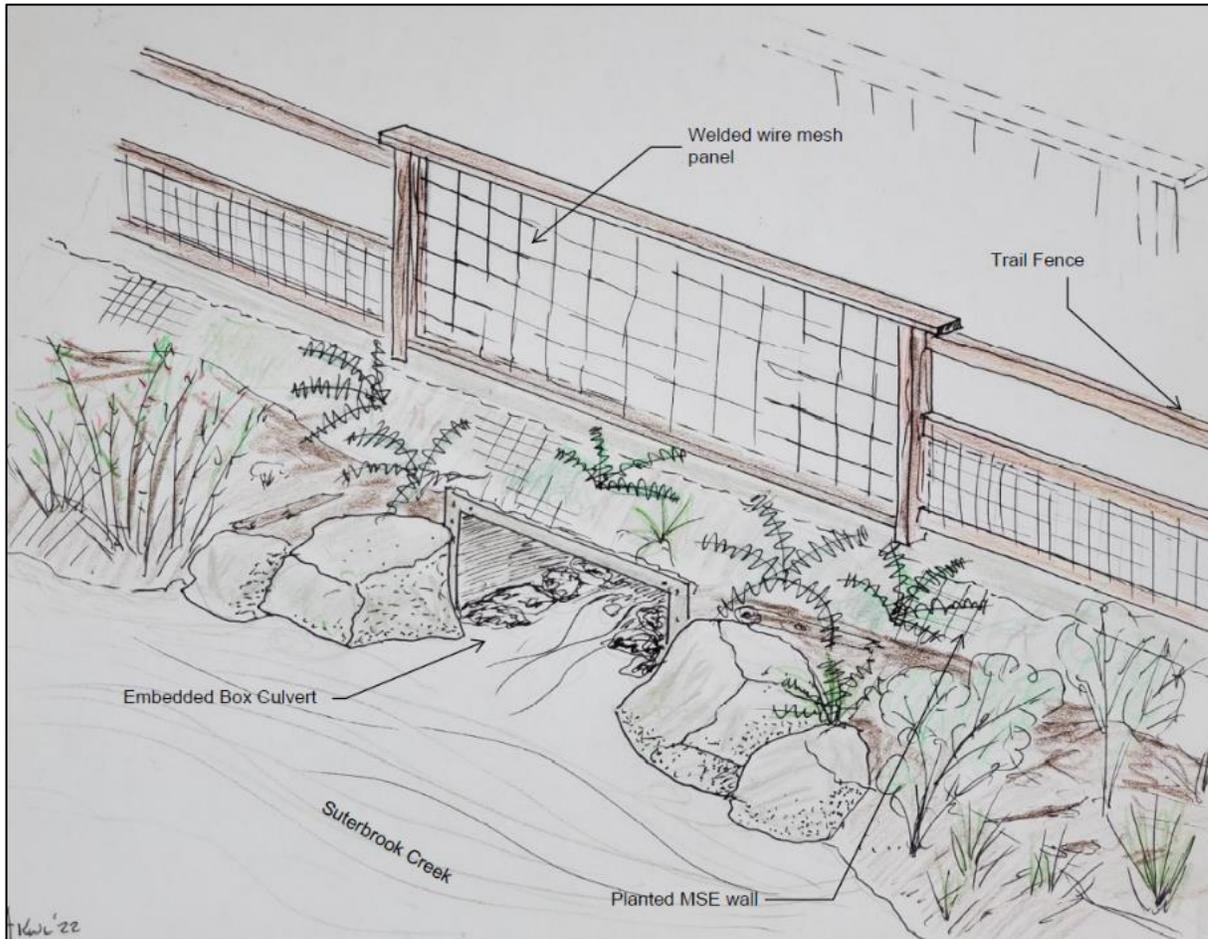
**Figure 7: Conceptual Rendering of Tributary Culvert and Wildlife Crossing**
