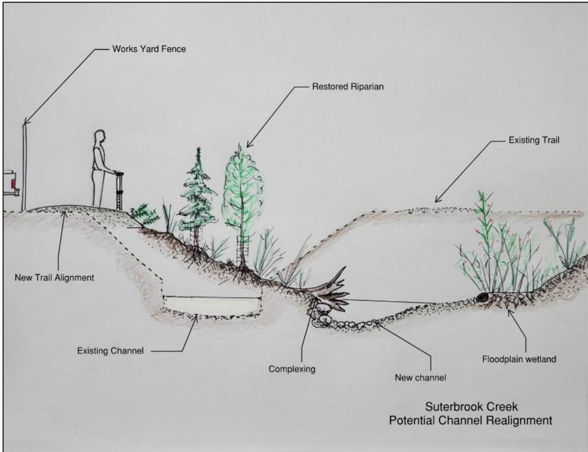
**Figure 10: Conceptual View of Suter Brook Mainstem Re-alignment**
