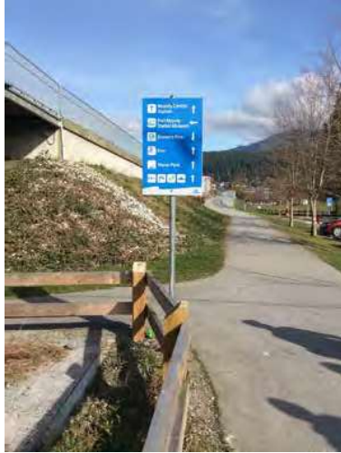
Directional sign with multiple destinations, Down arrows are confusing, Finger-post sign is a recommended solution. (See example on pages 64 & 65)
