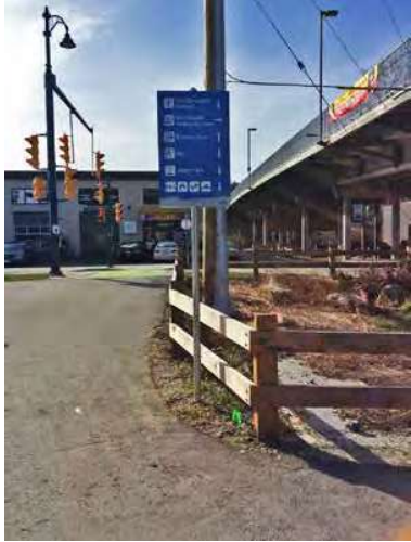
Directional sign with multiple destinations, Down arrows are confusing, Finger-post sign is a recommended solution. (See example on pages 64 & 65)
