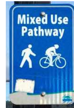
Typical regulatory sign, note pictograms are not in a white field and different from the versions provided.
