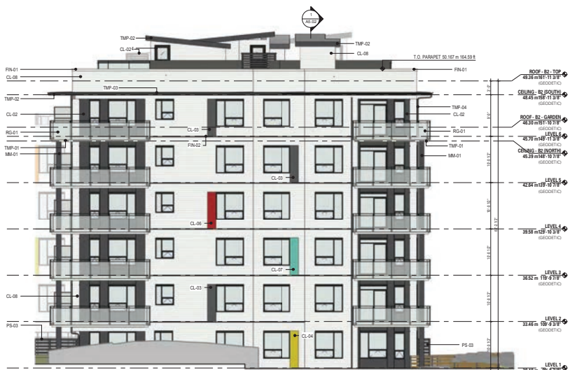
1 B2 - WEST ELEVATION (SOUTH) 1/8" = 1'-0"
