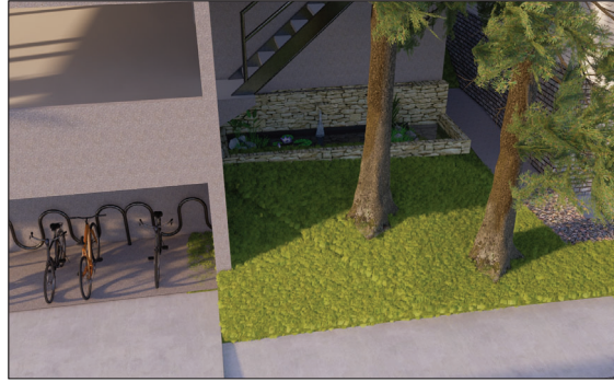
Water feature located at the lowest grade on site that collects rain water runoff from the site before draining it into the sewage network
