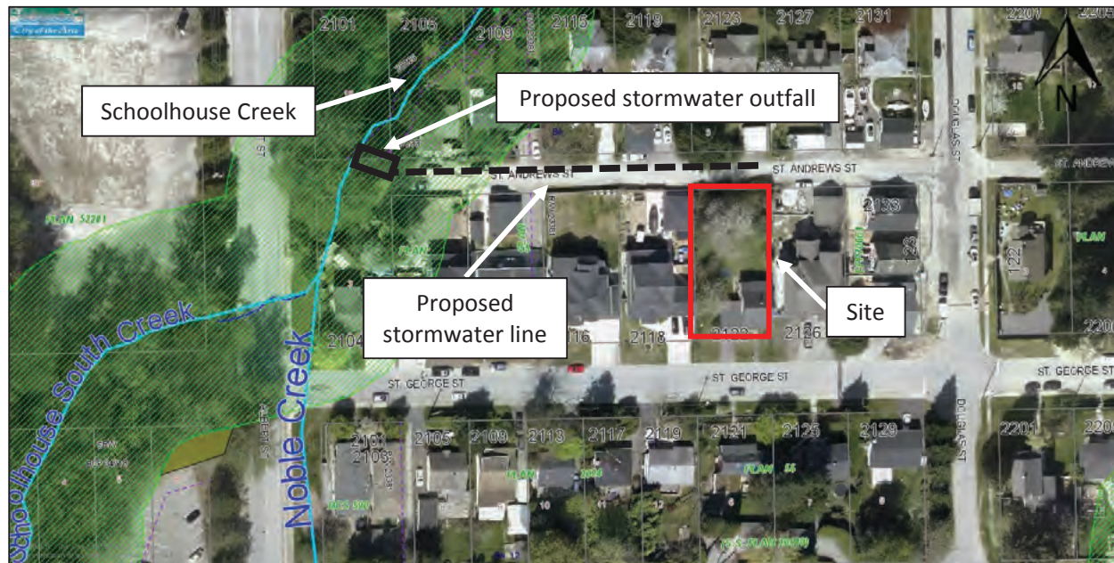
Figure 1: Site and Proposed Stormwater Infrastructure Location Overview.
